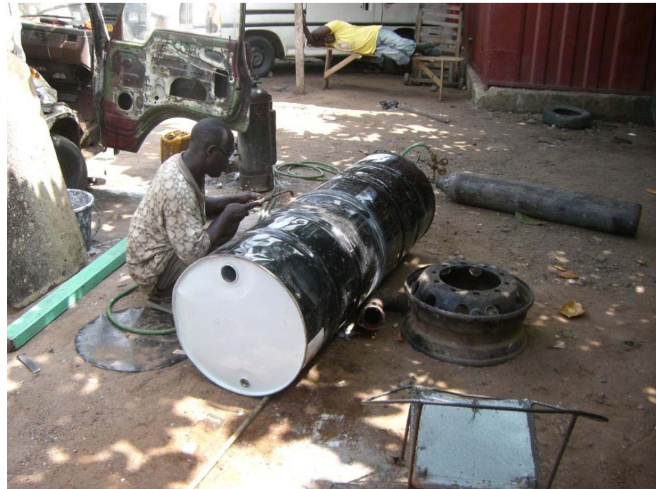
Welding 55 gallons drums into processor
